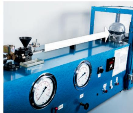
Impact testing equipment in the uvex testing center.
