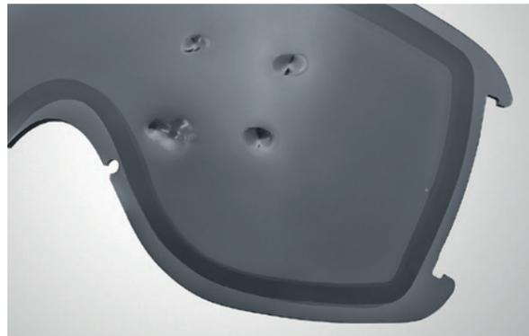
Dent in test lens after undergoing an impact test – the steel ball does not pass through the lens.
